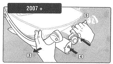
6 HOSE BRACKET / GAS CARTRIDGE SUPPORT BASKET REMOVAL
