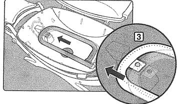
REASSEMBLY NOTE: Make sure that the igniter electrode opening is flush (touching) with the burner tube for proper ignition spark [3].
